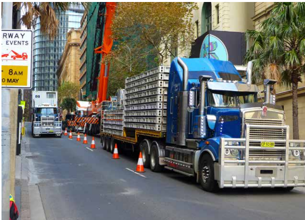
Figure 38: The use of dog-trailers is generally not supported. Any proposed usage requires the specific City approval .
