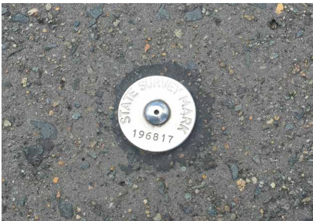
Figure 46: Examples of survey marks located in the City of Sydney LGA. Survey marks are important survey assets and are protected under legislation.
