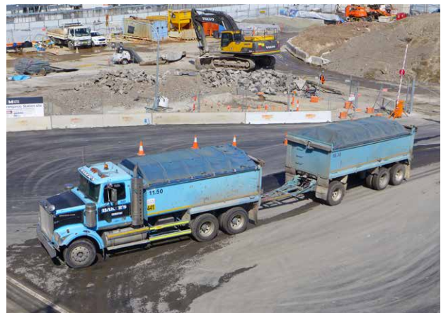
Figure 38: The use of dog-trailers is generally not supported. Any proposed usage requires the specific City approval .
