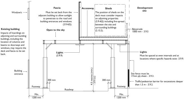
**Figure 58 (a) (top):** Section detail of a 'Type B' hoarding erected over a roadway. Potential impacts on adjoining properties and on vehicles including vehicle access to driveways must be considered in the design.
