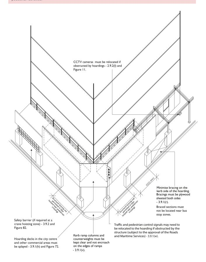
Figure 75: Design details for pedestrian ramps over concrete pump-lines (see Figure 73).
