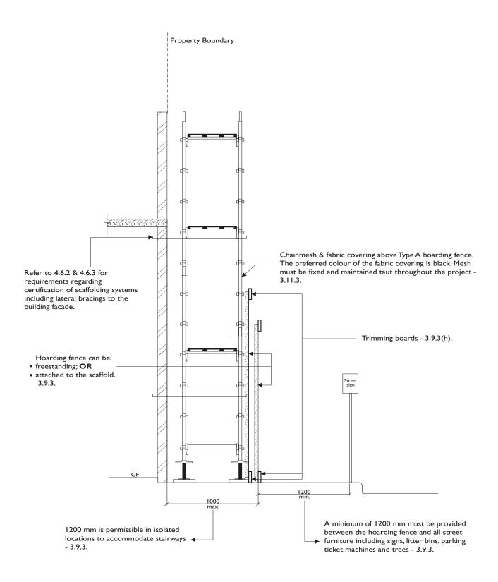
Figure 128: Elevation showing the key design features for scaffolding and 'Type A' hoardings.
